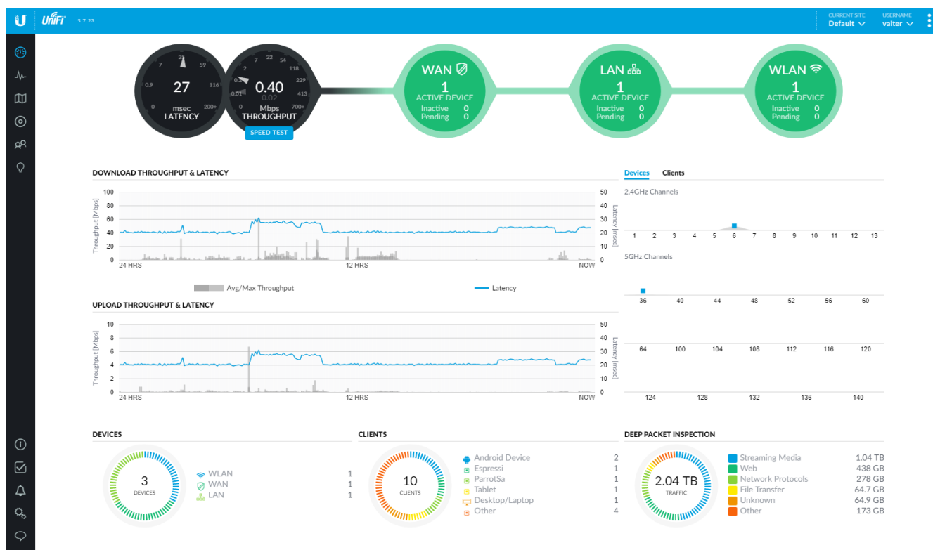
Figure 3.20: Example of the web interface of the Ubiquiti Unifi Cloud Key used at the Scandinavia Biogas Conference 2017.
