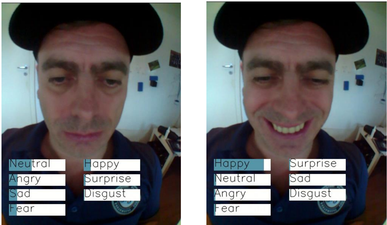
Figure 4.15: Images of the results of the test of the convolutional neural network on the video stream images using OpenCV and the Haar Cascades algorithm.
