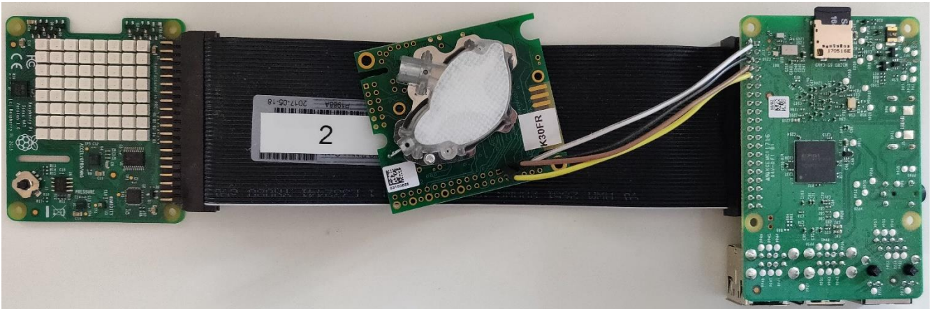
Figure 3.8: The final hardware solution for CO 2 , temperature, humidity and pressure measurements.
