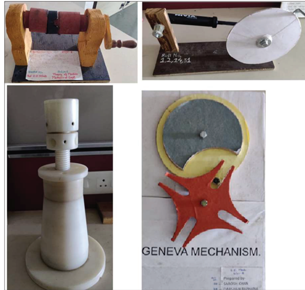
Figure 8 Mechanisms for course Theory of Machine.
