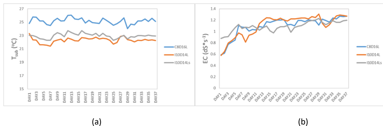
Figure 34. Average daily evolution of [a] substrate temperature ( T_{\text{sub}} in ^{\circ}\text{C} ) and [b] electric conductivity (EC in \text{dS}\cdot\text{s}^{-1} ) for healthy plants, i.e., C8D16L (the blue line), and stressed plants, i.e., I10D14L (the orange line) and I10D14Ls (the grey line). Days 1-37: a) C8D16L (control/continuous light), b) I10D14L (stress/normal intermittent light), and c) I10D14Ls (stress/shifting intermittent light).
